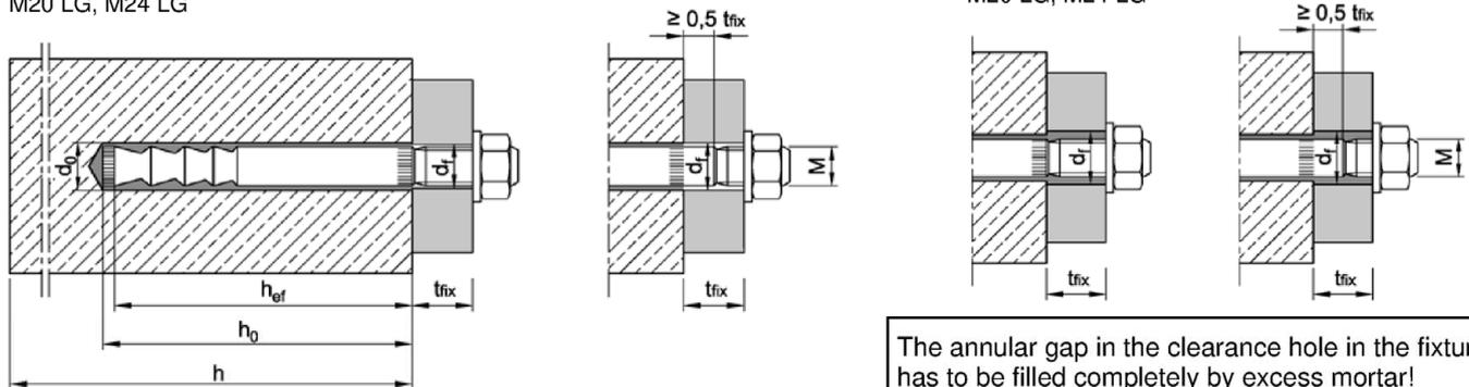
The annular gap in the clearance hole in the fixture has to be filled completely by excess mortar!
