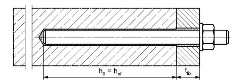
Pre-positioned or push through installation with subsequently injected filling disc (annular gap filled with mortar)
