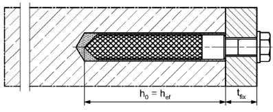
Pre-positioned installation with subsequently injected filling disc (annular gap filled with mortar)
