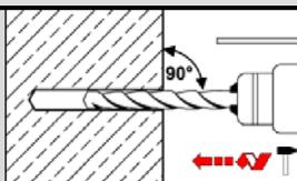
Drill the hole by applying the drilling method acc. to Annex B1, the drill bit diameter (Table B4) and the selected drill hole depth.
