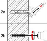
Starting from the bottom or back of the drill hole, blow the hole clean with the blow-out pump **four** times until retur air stream is free of noticeable dust.
