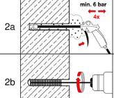
Starting from the bottom or back of the drill hole, blow out the hole with compressed air (min. 6 bar) **four** times, until return air stream is free of noticeable dust.
