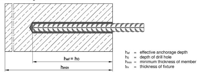
Injection system VMU plus for concrete
