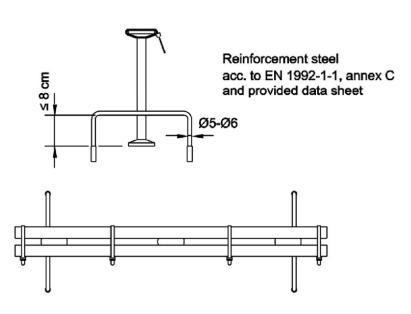
HALFEN HDB double headed studs for punching shear reinforcements
