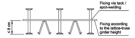
Fixing the HDB - reinforcing elements using spacers
