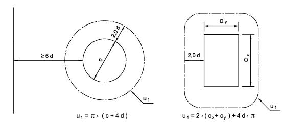
b) Loaded areas (columns) are less than 6d from openings (voids) in the slab.
