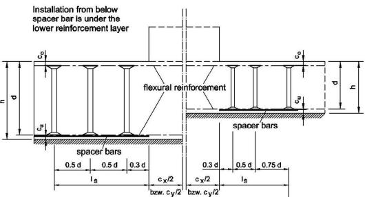
Concrete cover co resp. cu acc. to EN1992-1-1: 2004 + AC: 2010, section 4.4
