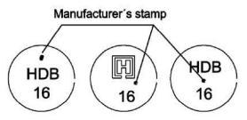
Material: reinforcement steel with a characteristic yield strength of  $f_{yk} \ge 500$  MPa acc. to EN 1992-1-1, annex C and provided data sheet
