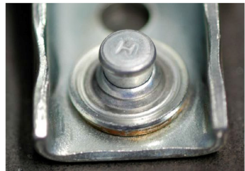
Clearly visible piston mark on top washer
