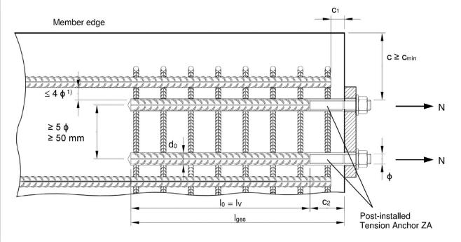
1) If the clear distance between lapped bars exceeds 4φ, then the lap length shall be increased by the difference between the clear bar distance and 4φ.
