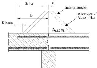
**Figure A2:** Overlapping joint at a foundation of a wall or column where the rebars are stressed in tension
