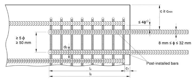
If the clear distance between lapped bars exceeds 4φ, then the lap length shall be increased by the difference between the clear bar distance and 4φ.
