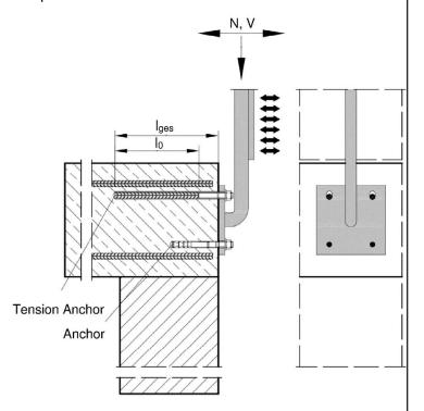
**Figure A8:** Overlap joint for the anchorage to centilever members
