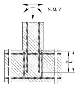
**Figure A4:** Rebar connection for components stressed primarily in compression. The rebars sre stressed in compression
