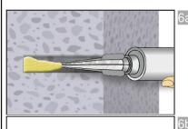
Starting from the bottom or back of the cleaned bore hole fill the hole with adhesive, until the level mark at the mixer extension (see below) is visible at the top of the hole. If the bottom or back of the anchor hole is not reached, an appropriate extension nozzle must be used. Slowly withdraw the static mixing nozzle and using a piston plugs during injection of the mortar, helps to avoid creating air pockets. Observe the gel-/ working times given in Table B3.
