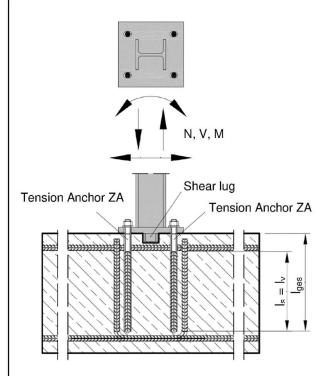
**Figure A7:** Overlap joint for the anchorage of barrier posts
