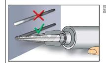
Prior to dispensing into the bore hole, squeeze out separately the mortar until it shows a consistent grey colour, but a minimum of three full strokes, and discard non-uniformly mixed adhesive components.
