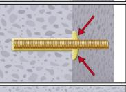
After inserting the anchor, the annular gab between anchor rod and concrete, in case of a push through installation additionally also the fixture, must be complete filled with mortar. If excess mortar is not visible at the top of the hole, the requirement is not fulfilled and the application has to be renewed.
