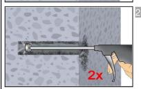
Finally blow the hole clean again with compressed air (min. 6 bar) (Annex B 4) a minimum of two times until return air stream is free of noticeable dust. If the bore hole ground is not reached an extension shall be used.
