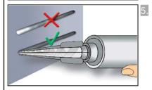
Prior to dispensing into the anchor hole, squeeze out separately a minimum of three full strokes and discard non-uniformly mixed adhesive components until the mortar shows a consistent grey colour.
