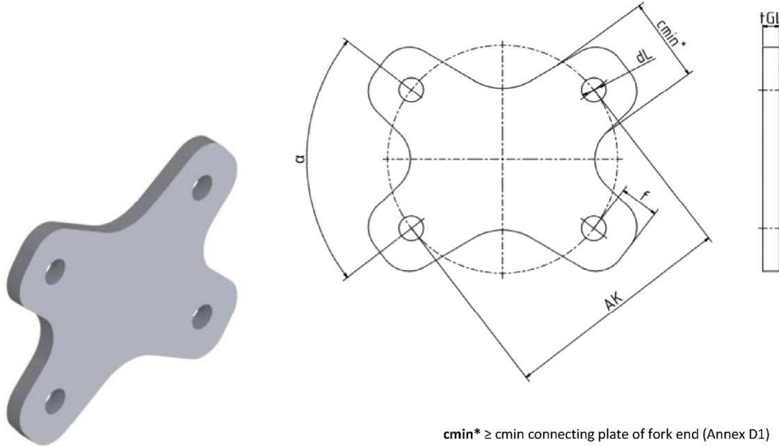
$cmin^* \geq cmin$  connecting plate of fork end (Annex D1)
