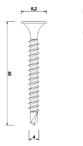
Dimensions in mm; Drawing without scale
