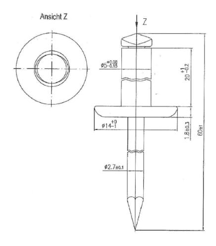
Dimensions in mm; Drawing without scale
