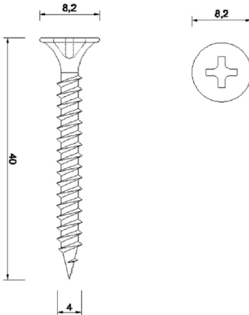
Dimensions in mm; Drawing without scale
