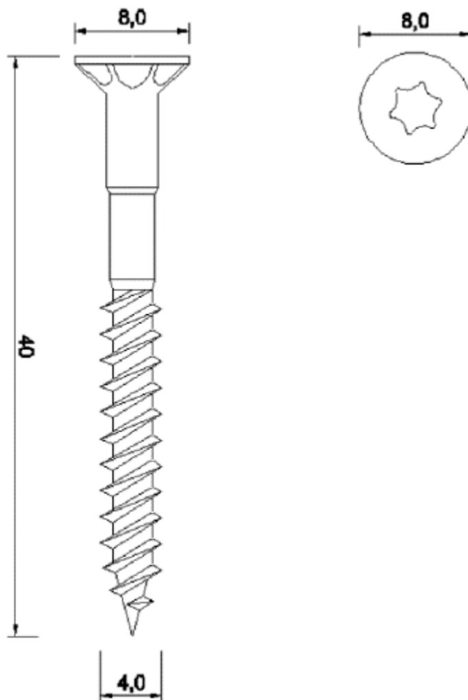
Dimensions in mm; Drawing without scale
