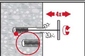
Brush 4 times with the specified brush (see Table B8) by inserting the steel brush Hilti HIT-RB to the back of the hole (if needed with extension) in a twisting motion and removing it. The brush must produce natural resistance as it enters the drill hole (brush  $\varnothing \geq$  drill hole  $\varnothing$ ) - if not the brush is too small and must be replaced with the proper brush diameter.
