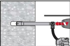
Drill hole to the required embedment depth with an appropriately sized Hilti TE-CD or TE-YD hollow drill bit attached to Hilti vacuum cleaner VC 20/40/60 or with a vacuum cleaner according to Table B8, in each case with automatic cleaning of the filter activated. This drilling system removes the dust and cleans the drill hole during drilling when used in accordance with the user's manual. After drilling is completed, proceed to the "injection preparation" step in the installation instruction.
