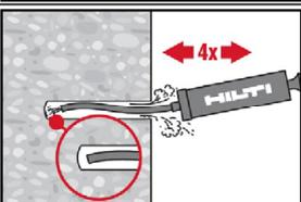
Blow out again with the Hilti hand pump at least 4 times until return air stream is free of noticeable dust.
