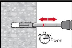
Before roughening water needs to be removed from the drill hole.
