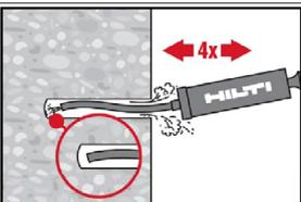
The Hilti hand pump may be used for blowing out drill holes up to diameters  $d_0 \leq 20$  mm and drill hole depths  $h_0 \leq 10 \cdot d$ .
