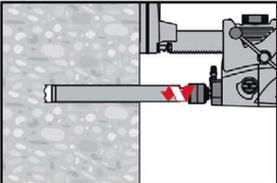
Diamond coring is permissible when suitable diamond core drilling machines and the corresponding core bits are used.
