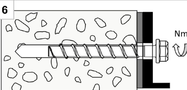
After adjustment, tighten the screw again
