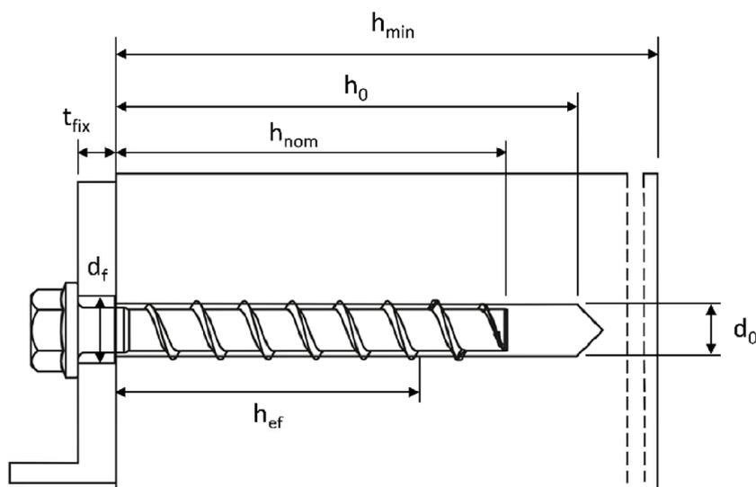
UIP ubolt concrete screw CSG-III
