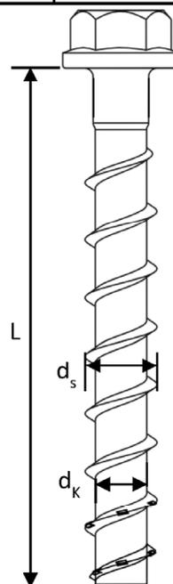
UIP ubolt concrete screw CSG-III
