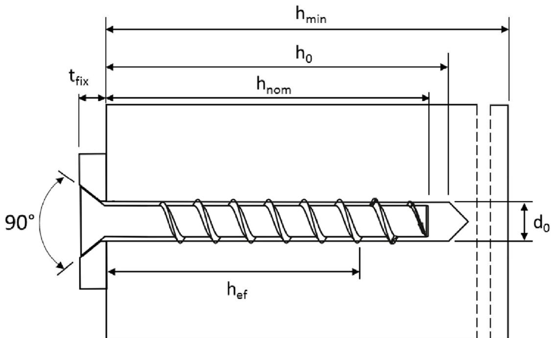
UIP ubolt concrete screw CSG-III
