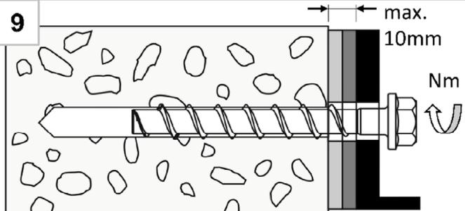
After adjustment, tighten the screw again
