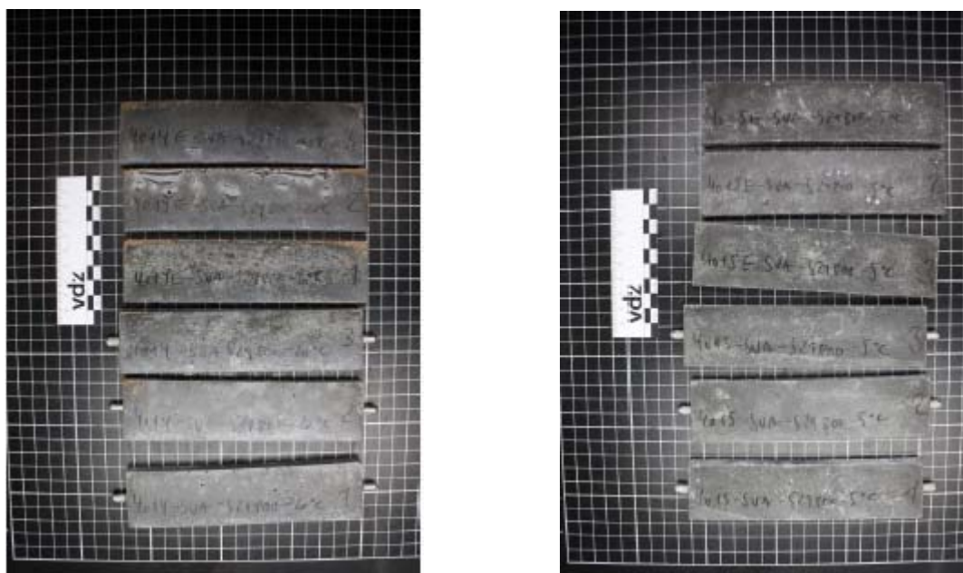
Figure A3: Specimens with CEM I 42,5 R-SR0 after sulfate storage; on the left: after 182 days at 20 °C; on the right: after 91 days at 5 °C
