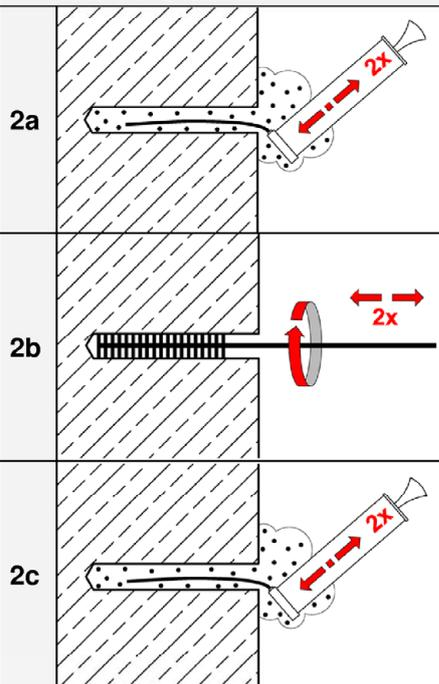
Blow out the drill hole completely at least **2x** from the bottom of the drill hole with blow-out pump or compressed air.
