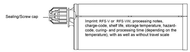
165 ml and 300 ml cartridge (Type: "foil tube")
