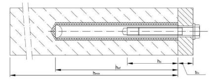
$t_{fix}$  = thickness of fixture
