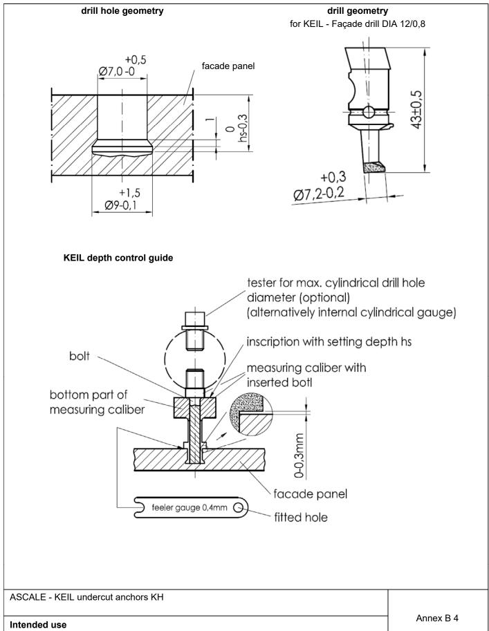
Drill hole dimensions Setting tools and testing equipment English translation prepared by DIBt
