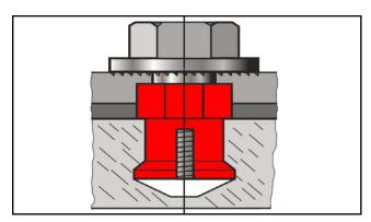
b) Installed anchor
