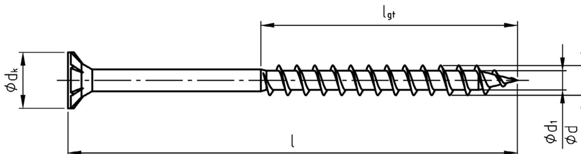
Partial thread without reamer shank and drilling tip/cutting edge
