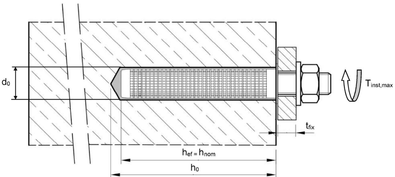
$h_{ef} = h_{nom}$  = effective anchorage depth
