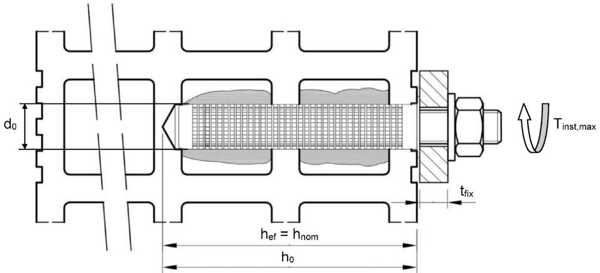
**Installation in solid brick; threaded rod and Internal threaded rod with or without sleeve**
