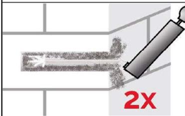
5c. Finally blow the hole clean again with handpump (Annex B4) a minimum of two times
