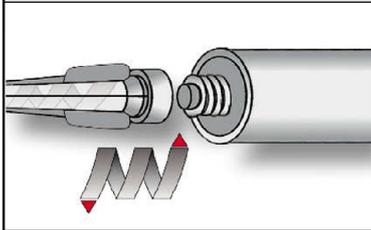
1. Remove the cap and attach the supplied static-mixing nozzle to the cartridge and load the cartridge into the correct dispensing tool. In case of a foil tube cartridge, cut off the clip before use. For every working interruption longer than the recommended working time (Table B4 and B5) as well as for new cartridges, a new static-mixer shall be used.
