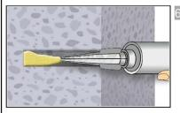
Starting from the bottom or back of the cleaned anchor hole, fill the hole up to approximately two-thirds with adhesive. Slowly withdraw the static mixing nozzle as the hole fills to avoid creating air pockets. If the bottom or back of the anchor hole is not reached, an appropriate extension nozzle must be used. Observe the gel-/ working times given in Table B4.
