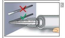
Prior to dispensing into the anchor hole, squeeze out separately a minimum of three full strokes and discard non-uniformly mixed adhesive components until the mortar shows a consistent grey or red colour.
