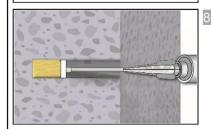
Insert piston plug to back of the hole and inject adhesive. If the bottom or back of the anchor hole is not reached, an appropriate extension nozzle must be used.
