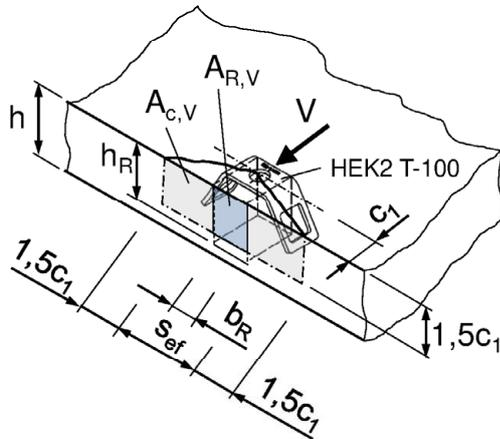
$$A_{c,V} = (3c_1 + s_{ef}) \cdot 1,5c_1 - A_{R,V} \quad (11)$$
