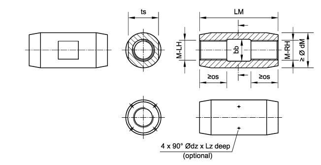
Minimum screw-in length of the tension rod = om - oj according to Annex B3
