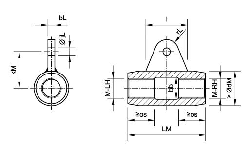
Minimum screw-in length of the tension rod = om - oj according to Annex B3 \* /.. alternative dimensions for a M10 tension rod connection
