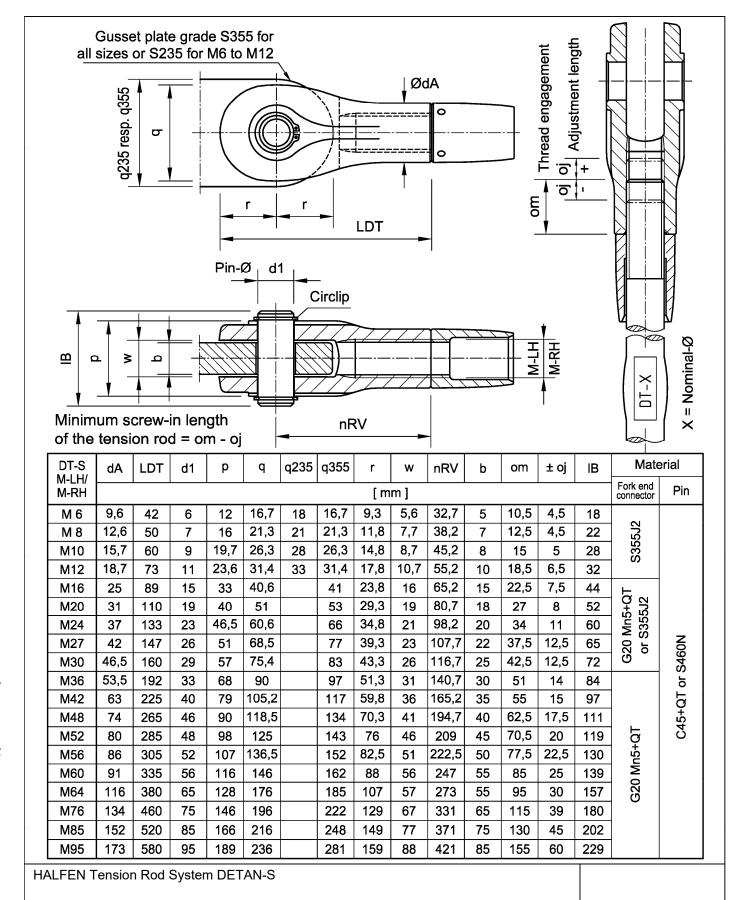
Dimensions of the fork end connector and minimum dimensions of the gusset plates
