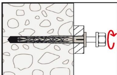
4. The screw is screwed-in until the head of the screw touches the sleeve. The anchor is correctly mounted, when the head of the screw fits tight on the surface and cannot be screwed-in any further.
