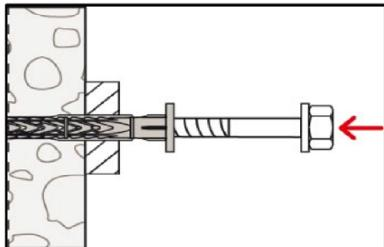
3. Insert anchor (screw and sleeve) by using a hammer until the collar of the plastic sleeve is flush with the surface of the fixture. In case of using brick S8 (see Table A3.1 footnote 4), additional embedment depths  $h_{nom}$  150mm or  $h_{nom}$  180 mm may be taken by measuring the anchorage depth and the fixture height. The corresponding length of anchor should be taken.
