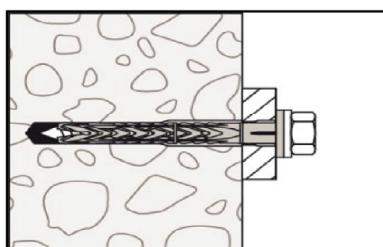
5. Correctly installed anchor in concrete.
