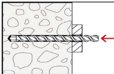
1. Drill the bore hole according to Table B3.1 using the drilling method described in the corresponding Annex C.
