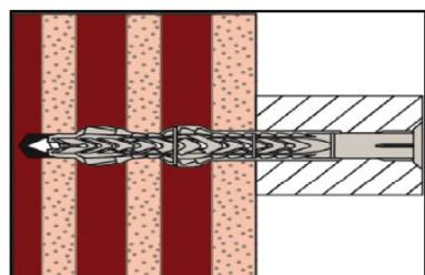
6. Correctly installed anchor in hollow or perforated masonry.
