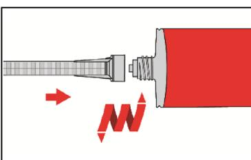
3. Screw on static-mixing nozzle SM-14W/PM-19E and load the cartridge into an appropriate dispensing tool. With foil tube cartridges cut off the foil tube clip before use.
