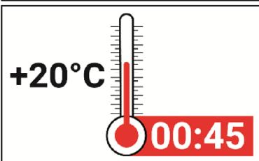
12. Temperature related curing time  $t_{cure}$  (Annex B 5) must be observed. Do not move or load the fastener during curing time.
