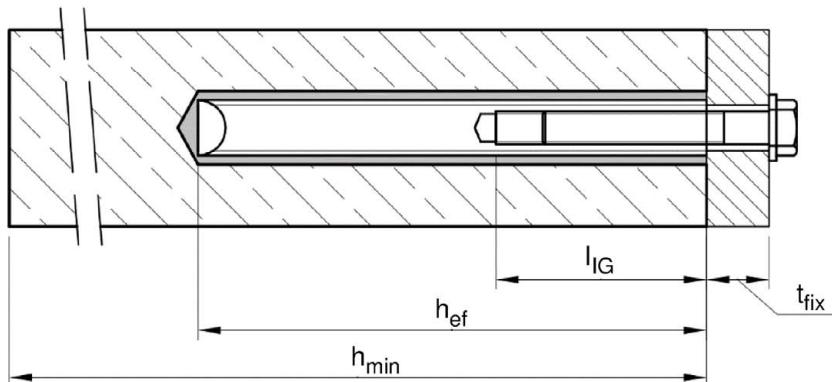
$t_{fix}$  = thickness of fixture
