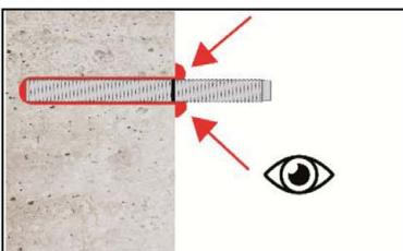
10. Annular gap between anchor rod and base material must be completely filled with mortar. In case of push through installation the annular gap in the fixture must be filled with mortar also. Otherwise, the installation must be repeated starting from step 7 before the maximum working time  $t_{work}$  has expired.
