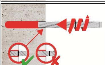
9. Insert the anchor rod while turning slightly up to the embedment mark.
