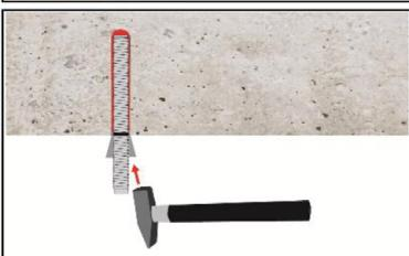
11. For application in vertical upwards direction the anchor rod shall be fixed (e.g. wedges).
