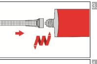
Screw on static-mixing nozzle SM-14W/PM-19E and load the cartridge into an appropriate dispensing tool. With foil tube cartridges cut off the foil tube clip before use.
