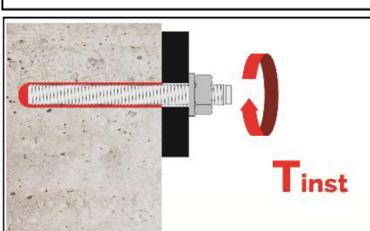
12. Install the fixture by using a calibrated torque wrench. Observe maximum installation torque (Table B1, B2 or B3). In case of static requirements (e.g. seismic), fill the annular gap in the fixture with mortar (Annex A 3). Therefore replace the washer by the filling washer VFS and use the mixer reduction nozzle MR.
