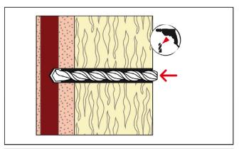
1. Drill hole by corresponding drilling method defined for each stone according to Table C1.1 and drill hole diameter d₀ and depth h₁ according to Table B2.1.
