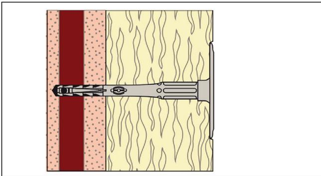
1. Drill hole by corresponding drilling method defined for each stone according to Table C1.1 and drill hole diameter  $d_0$  and depth  $h_1$  according to Table B2.1.
