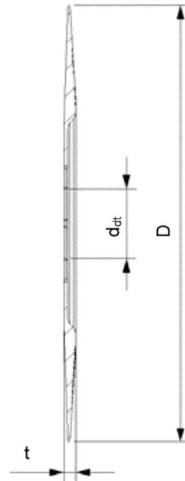
**Table A3.2: Slip-on plate, dimensions and material**
