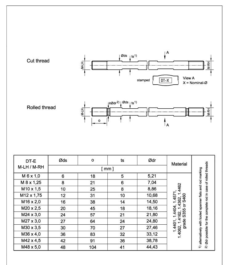
HALFEN Tension Rod System DETAN-E
