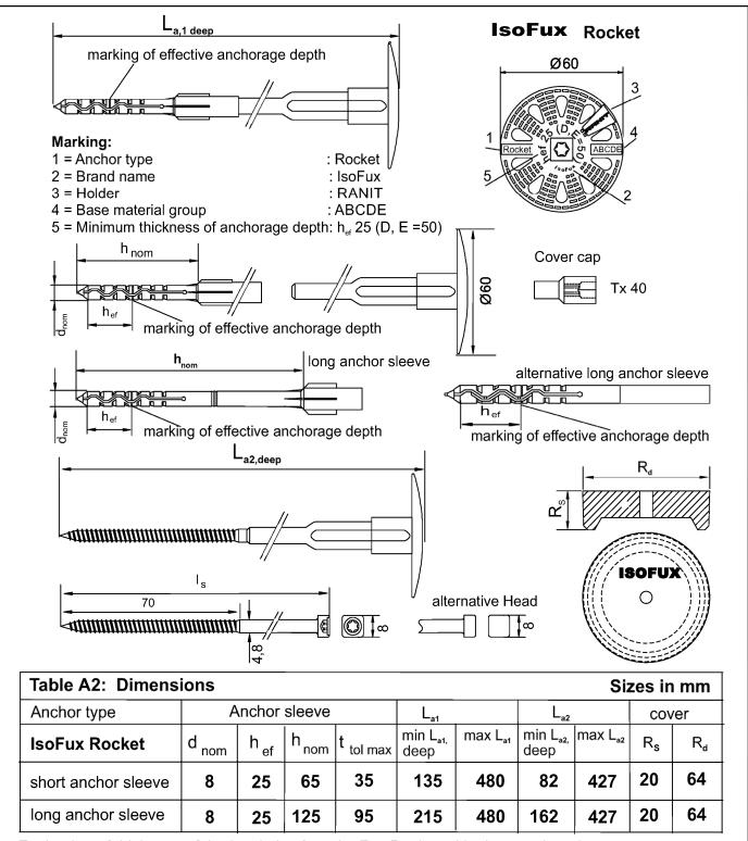
Evaluation of thickness of the insulation  $h_{Dmax}$  IsoFux Rocket with short anchor sleeve min  $L_{a1, deep}$  - h  $_{nom}$  - 30 + Rs =  $h_{Dmax}$ ; e.g.: (min  $L_{a1, deep}$  = 155) 155 -65 -30 +20 = 80 ( $h_{Dmax}$ )
