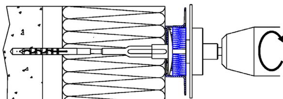
5) Anchor with the screw drill mounting. The bottom side of the plate must be flush with the ETICS.
