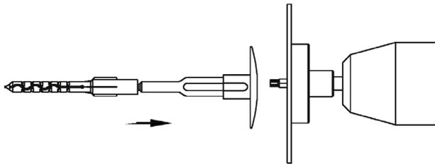
2) Put the anchor on the mounting tool.
