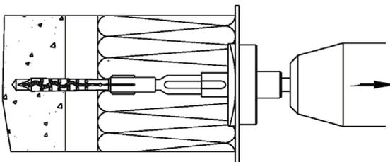
5) Installed condition. remove the mounting tool.
