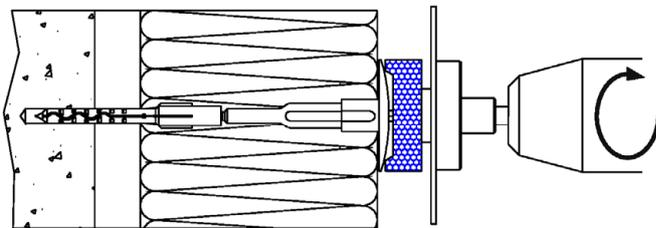
4) Anchor with the screw drill mounting. The bottom side of the plate must be flush with the ETICS.
