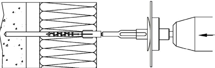
3) Place the anchor into the drill hole.
