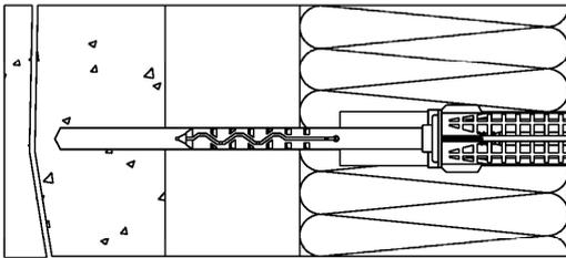
2) Put the EVO stick into the hole. Insert the EVOLution screw-in tool. Fix the EVO stick with the EVOLution setting tool until the „Distance Control“ (= The marked orange sleeve )
