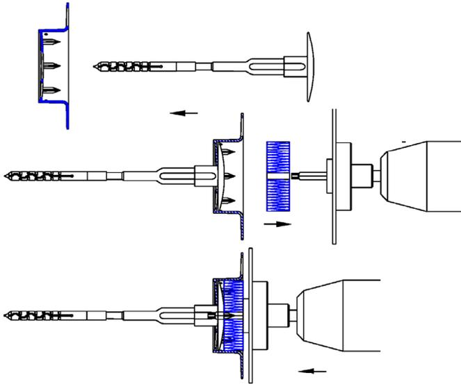
2) Put the anchor IsoFux Rocket in the MW-CUP
