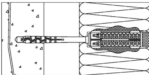
4) Gluing the dowel including foaming the adhesive channel. Cut the dried-out adhesive foam flush with a knife.
