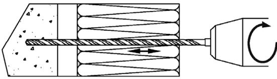
1) Drill the hole perpendicular to the substrate surface.
