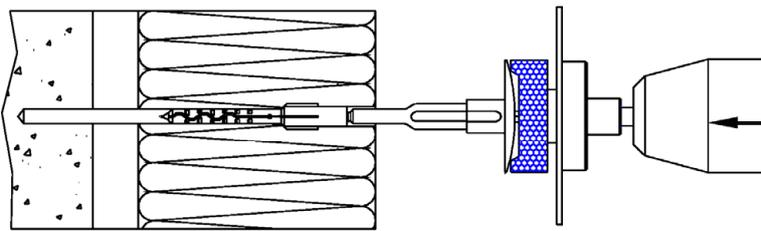
3) Place the anchor into the drill hole.
