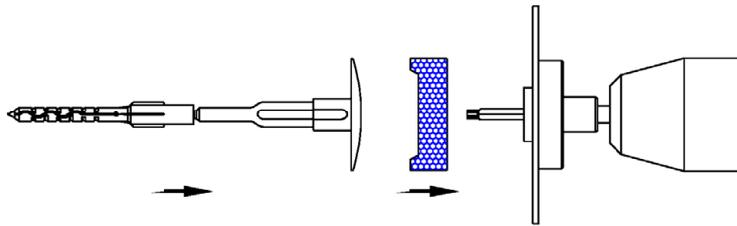
2) Put the anchor and the insulation cover on the mounting tool.
