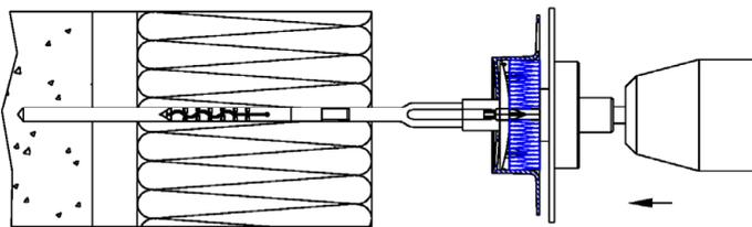
4) Place the anchor into the drill hole.
