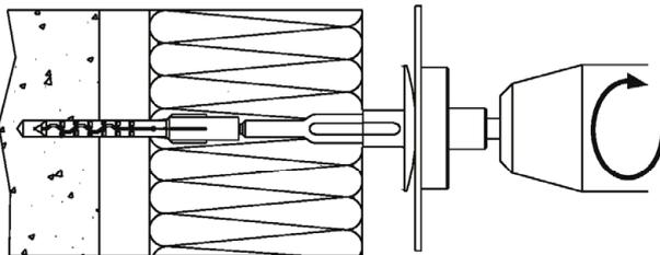
4) Anchor with the screw drill mounting. The bottom side of the plate must be flush with the ETICS.
