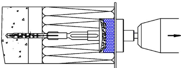
5) Installed condition. remove the mounting tool.
