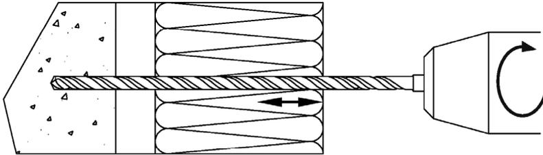
1) Drill the hole perpendicular to the substrate surface. Clean the drill hole.
