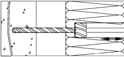
1) Drill the hole with EVOLution drill perpendicular to the surface. Clean the drill hole.
