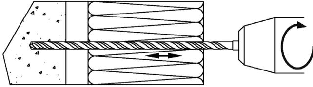
1) Drill the hole perpendicular to the substrate surface. Clean the drill hole.
