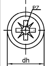
cylinder with small countersunk head
