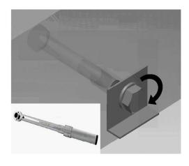
Apply installation torque with the help of a torque wrench. T<sub>inst</sub> must not be exceeded.
