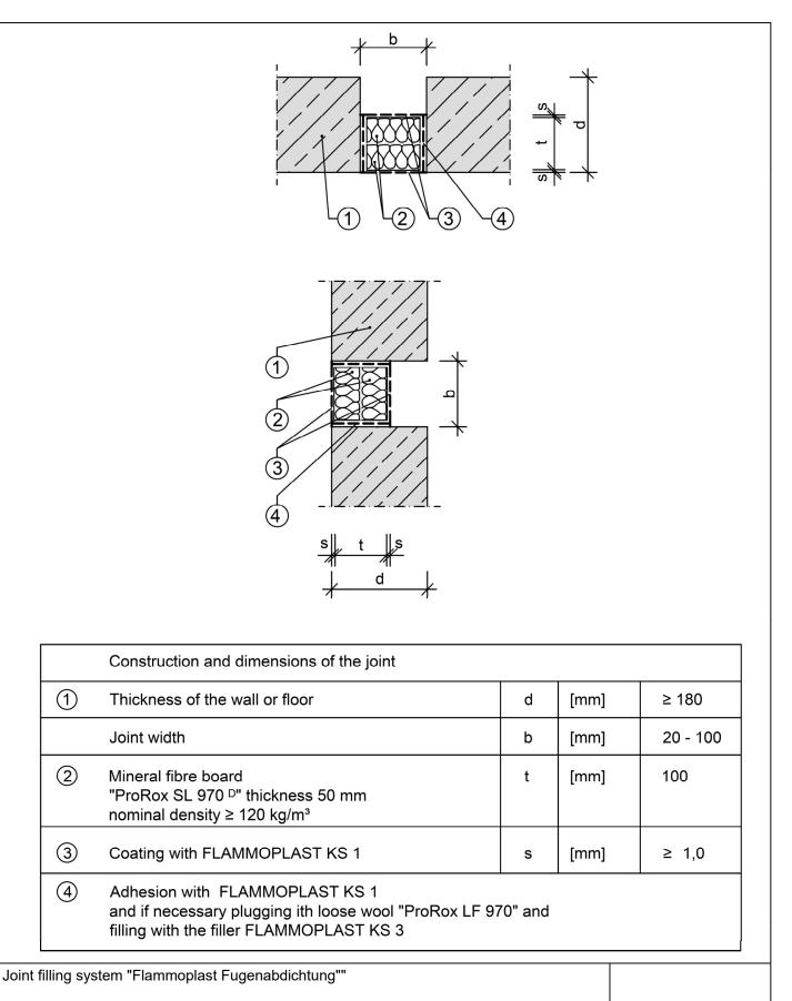
Resistance to fire of the joint filling system - use in floors and walls - Annex B3
