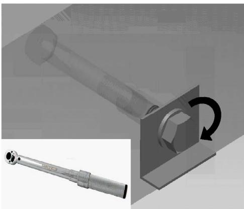
Apply installation torque with the help of a torque wrench.
