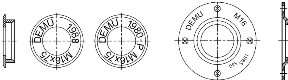
Data clip: section and top view (with example for marking)
