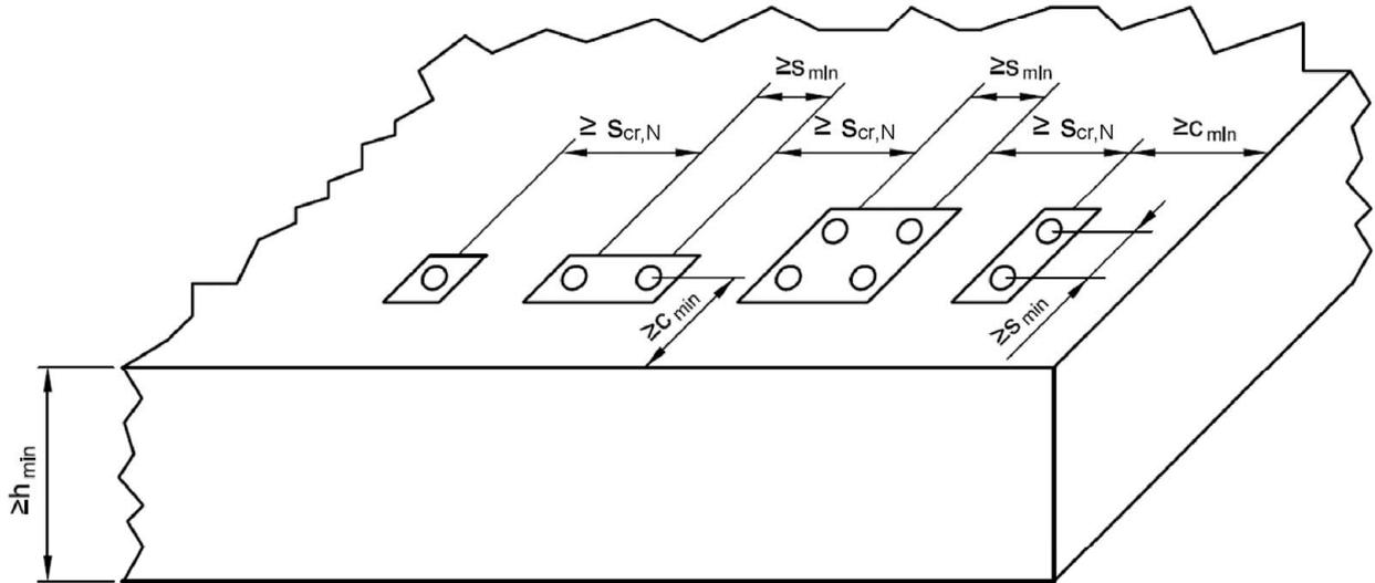
The mentioned spacings, edge distances and member thicknesses apply also for anchors installed in the front edge.
