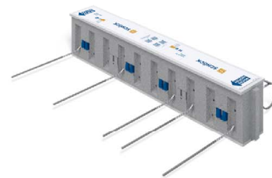
Fig. A.6: Schöck Isokorb® Type Q for supported balconies, for example shear force bar with bent bar end on the ceiling side (alternatively with straight bar end on the ceiling side)
