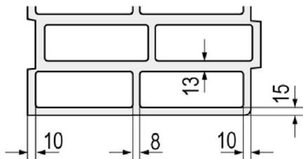
Vertical perforated brick HLz, EN 771-1:2011+A1:2015; e.g. Ziegelwerk Brenner according to Annex C 24
