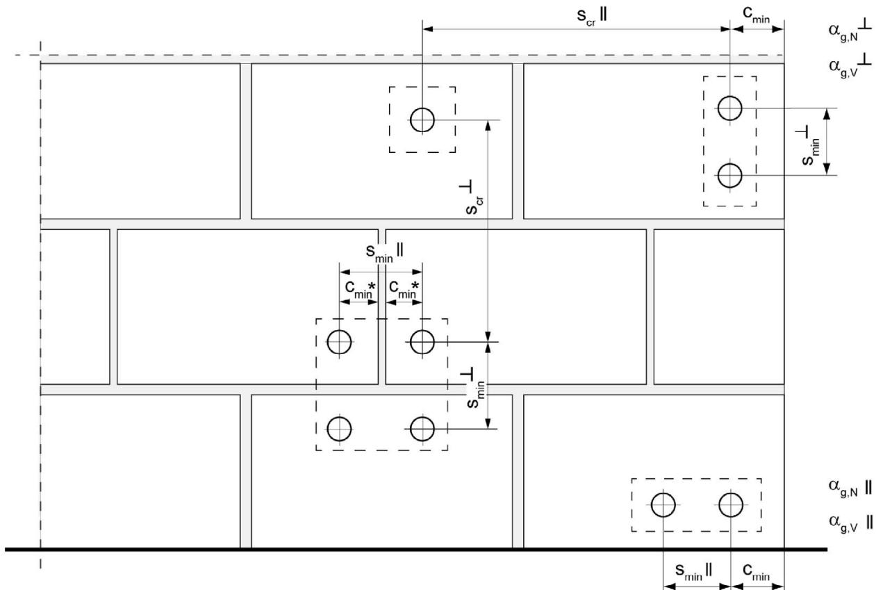
\* Only, if vertical joints are not completely filled with mortar
