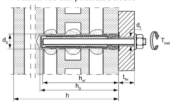
Internal threaded anchor with perforated sleeve
