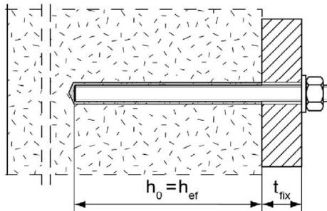
**Push through anchorage: Annular gap filled with mortar**
