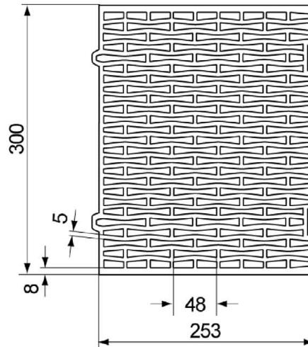
Vertical perforated brick HLz, Porotherm W 44, filled with mineral wool, EN 771-1:2011+A1:2015 according to Annex C 26
