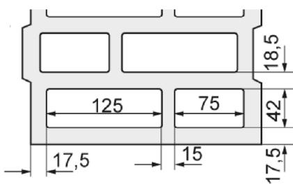
Light-weight concrete hollow block Hbl, EN 771-3:2011+A1:2015; according to Annex C 28
