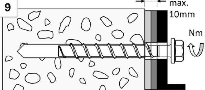
After adjustment, tighten the screw again
