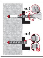
Find the thread in the drilled hole
