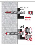
A screw can get adjusted maximum two times. The total allowed maximum thickness of shims added during the adjustment process is 10 mm. The final embedment depth after adjustment process must be larger or equal than  $h_{\text{nom}}$ .
