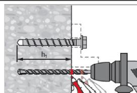
Mark drilling depth  $h_1$  for pre or through installation.
