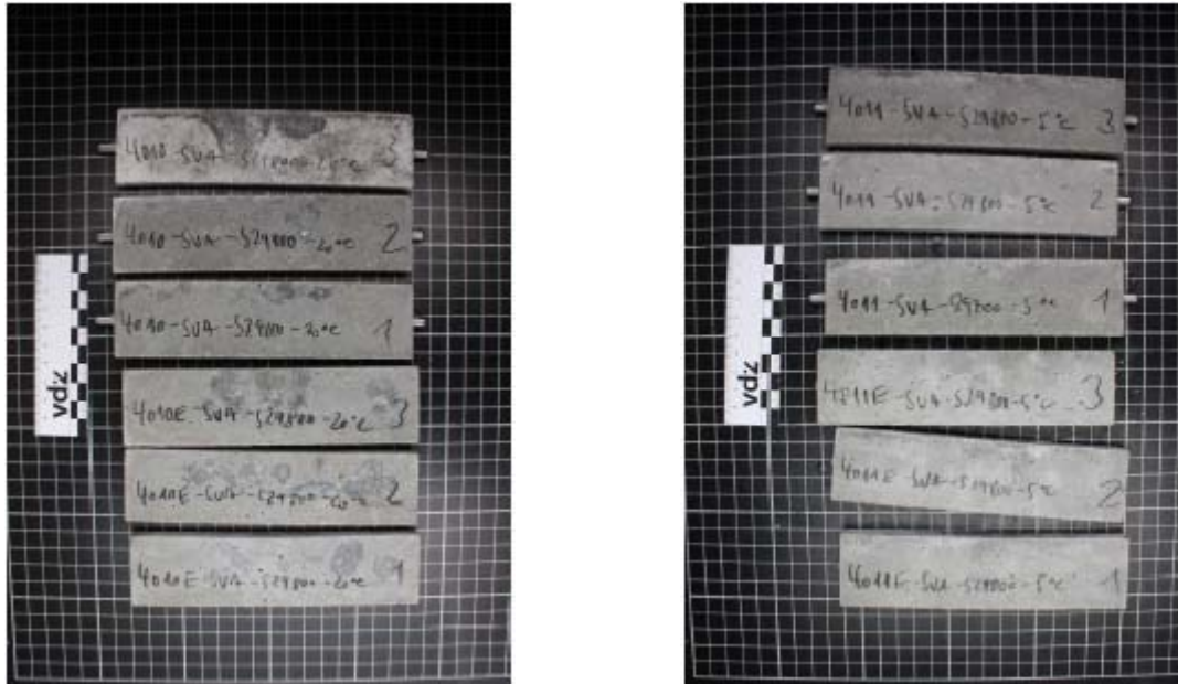
Figure A1: Specimens with CEM III/A XX-LH/SR/LA "Eisenhüttenstadt" after sulfate storage; on the left: after 182 days at 20 °C; on the right: after 91 days at 5 °C
