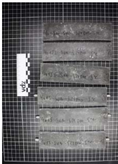
Figure A3: Specimens with CEM I 42,5 R-SR0 after sulfate storage; on the left: after 182 days at 20 °C; on the right: after 91 days at 5 °C
