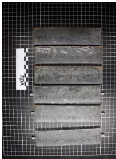
Figure A3: Specimens with CEM I 42,5 R-SR0 after sulfate storage; on the left: after 182 days at 20 °C; on the right: after 91 days at 5 °C
