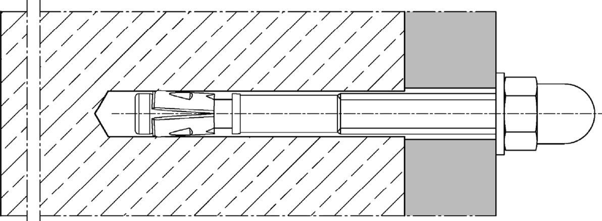
Wedge Anchor AN BZ3 / AN BZ3 A4 / AN BZ3 HCR
