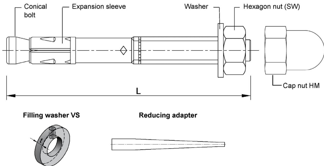
**Wedge Anchor AN BZ3 / AN BZ3 A4 / AN BZ3 HCR**
