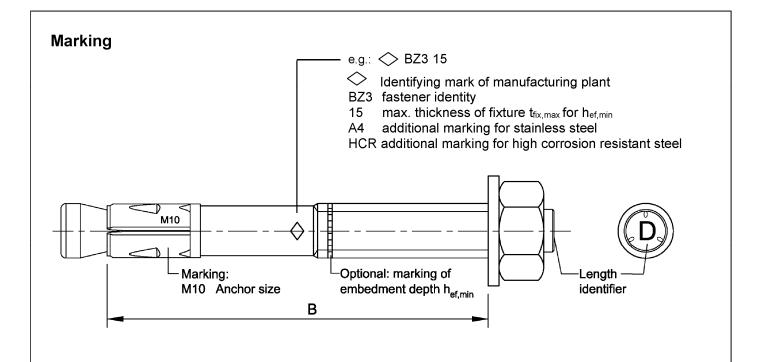
Usable length:  $B = h_{ef} + t_{fix}$
