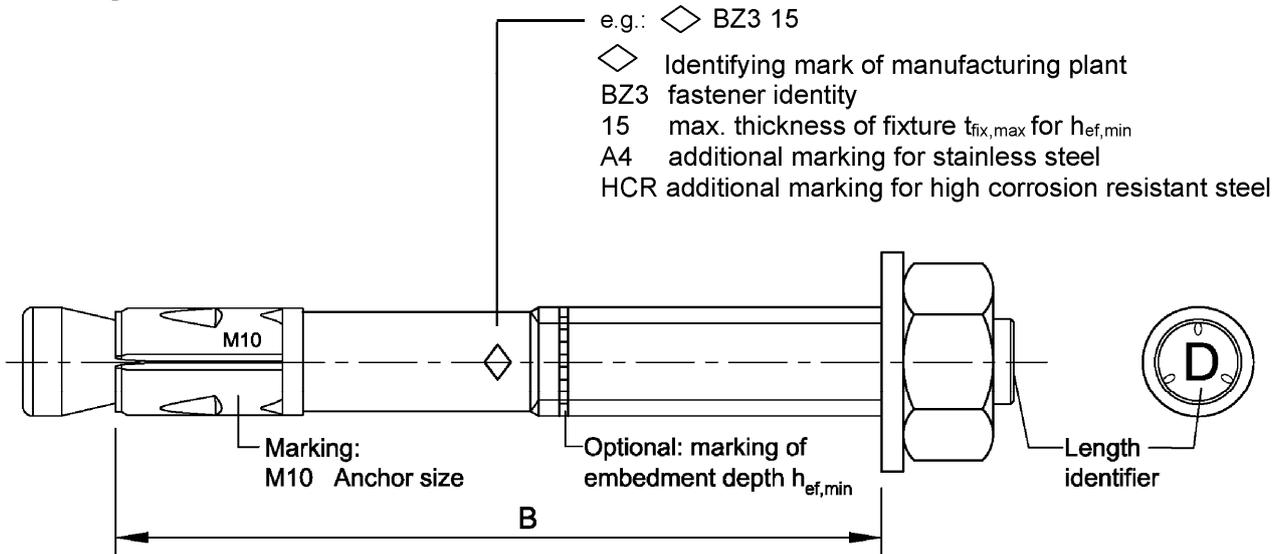
Usable length:  $B = h_{ef} + t_{fix}$
