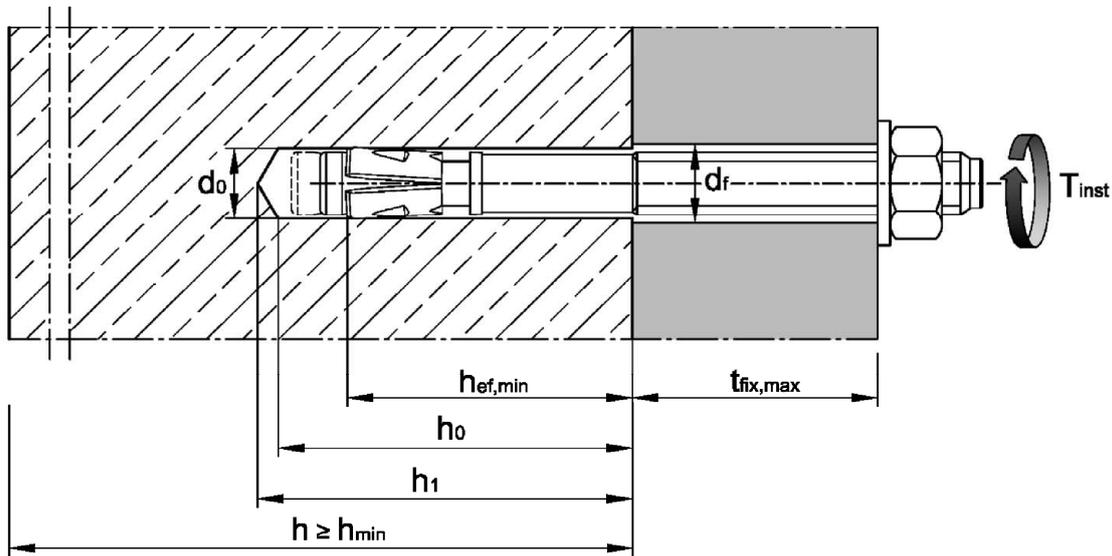
**Wedge Anchor AN BZ3 / AN BZ3 A4 / AN BZ3 HCR**
