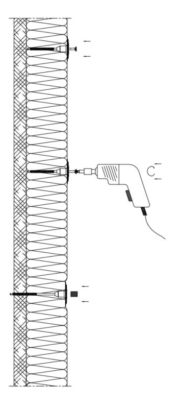
Push the anchor into the insulation material until the plate flushes with the insulation board surface.
