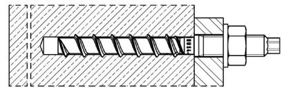
HUS4-A (threaded rod connection sizes 10 with M12 and 14 with M16)
