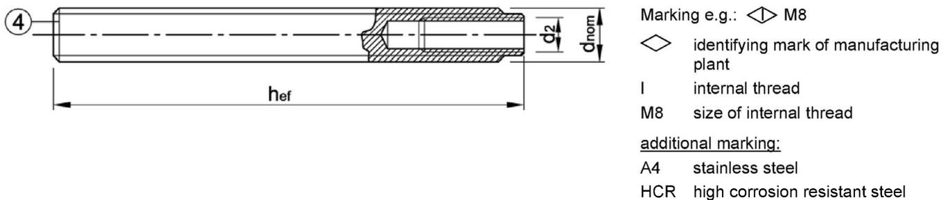
**Injection System VME basic for concrete**
