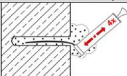
Starting from the bottom or back of the drill hole, blow out the hole with the blow-out pump a minimum of **four** times until return air stream is free of noticeable dust.
