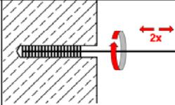
Check brush diameter (Table B4). Brush the hole with an appropriate sized wire brush  $\geq d_{b,min}$  (Table B4) a minimum of **two** times. If the drill hole ground is not reached with the brush, an appropriate brush extension must be used.
