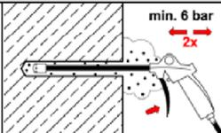
Starting from the bottom or back of the drill hole, blow out the hole with compressed air (min. 6 bar) a minimum of **two** times until return air stream is free of noticeable dust. If the drill hole ground is not reached, an extension must be used.
