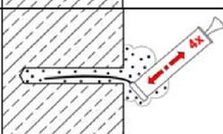
Starting from the bottom or back of the drill hole blow out the hole again a minimum of **four** times until return air stream is free of noticeable dust.
