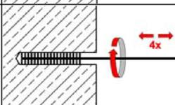
Check brush diameter (Table B4). Brush the hole with an appropriate sized wire brush  $\geq d_{b,min}$  (Table B4) a minimum of **four** times. If the drill hole ground is not reached with the brush, an appropriate brush extension must be used.
