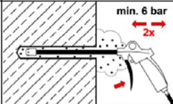
Starting from the bottom or back of the drill hole, blow out the hole with compressed air (min. 6 bar) again a minimum of **two** times until return air stream is free of noticeable dust. If the drill hole ground is not reached, an extension must be used.
