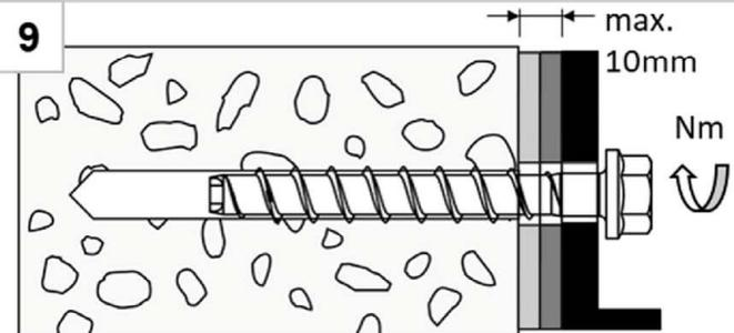
After adjustment, tighten the screw again
