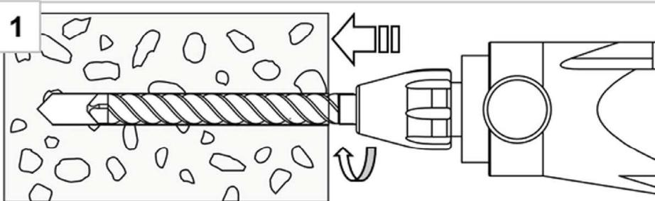
Create hammer drilled or hollow drilled borehole
