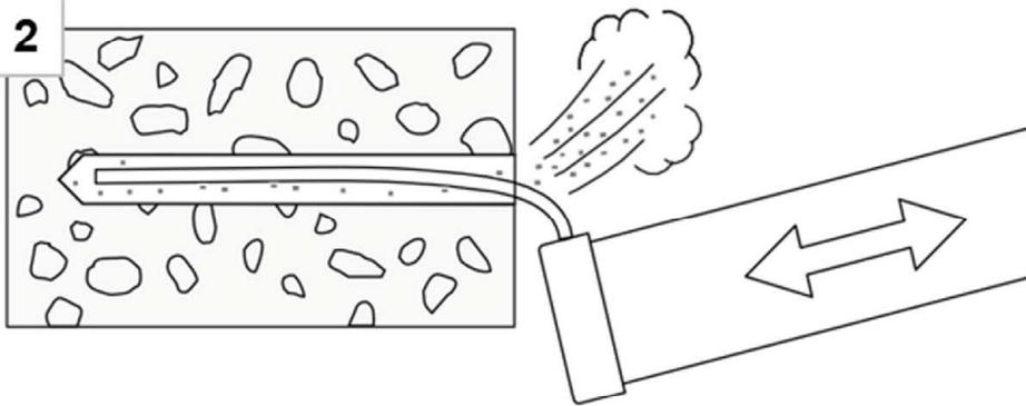
Remove drill dust by vacuuming or blowing of
