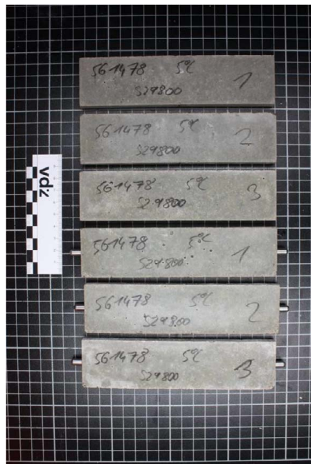
Figure A2: Specimens with CEM III/B 32,5 N-LH/SR after sulfate storage; on the left: after 182 days at 20 °C; on the right: after 91 days at 5 °C
