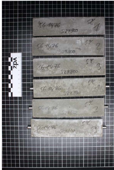
Figure A1: Specimens with CEM III/A 32,5 N-LH/SR/LA "Lägerdorf" after sulfate storage; on the left: after 182 days at 20 °C; on the right: after 91 days at 5 °C
