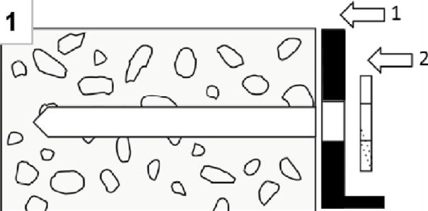
After preparing borehole (Annex B5, figure 1+2), position first fixture (1), than filling washer (2)
