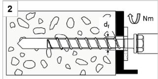
Install with torque impact screw driver or torque wrench
