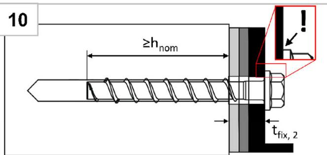
The head must be undamaged and in contact with the fixture
