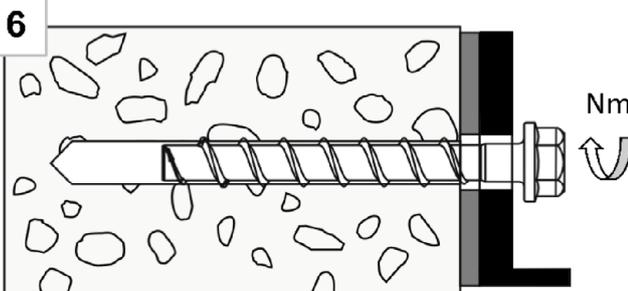
After adjustment, tighten the screw again
