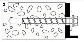
Installed condition without injected mortar in the filling washer
